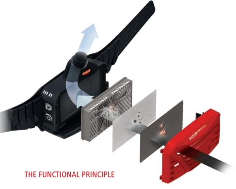
The fresh air system consists of a fresh air blower, interconnecting hose and carrying strap. The fresh air blower attached to the carrying strap filters up to 99.8% of welding fume particles out of the ambient air via a TH3 particle filter (highest possible classification) and directs the cleaned air directly into the Vizor Connect via the interconnecting hose. This represents an almost 100 percent improvement in terms of exposure to welding fume particles.
