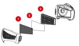
1 Spark arrestor to block coarse powders.
