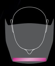
Expanded field of view with a flat filter requires a wider helmet.
