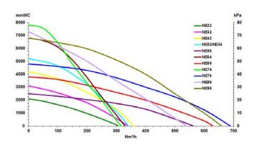
Air Powered ejectors
