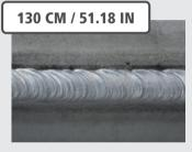
Material: CrNi Material thickness: 6 mm / 0.24 in I: 150 A Gas: Argon
