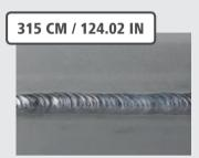
Material: CrNi Material thickness: 2 mm / 0.08 in I: 82 A Gas: Argon
