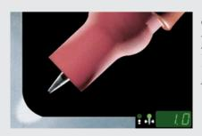
Cap diameter: 1 mm Base metal: AIMg3 Sheet thickness: 5 mm Welding amperage: 185 A Welding voltage: 15.6 V AC balance: -5
