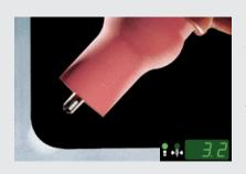
Cap diameter: 3.2 mm Base metal: AIMg3 Sheet thickness: 5 mm Welding amperage: 185 A Welding voltage: 15.6 V AC balance: 0
