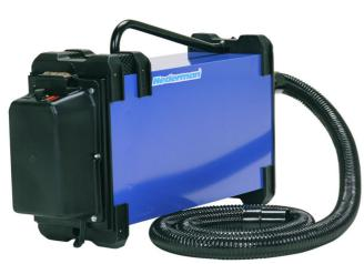
The Fume Eliminator is designed to be carried to the working area. Connected to a welding torch or to an extraction nozzle, the FE unit extracts the fume directly at source. FE 840 has a manual start/stop function while the FE 841 has an automatic start/stop function, which starts the unit as soon as the welding begins.
