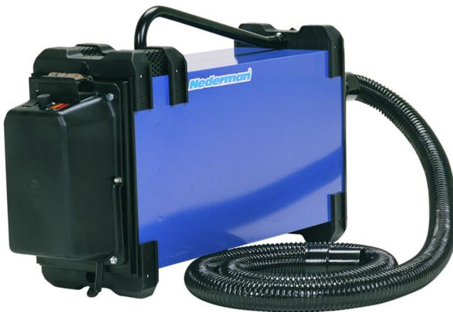
The Fume Eliminator is designed to be carried to the working area. Connected to a welding torch or to an extraction nozzle, the FE unit extracts the fume directly at source. FE 840 has a manual start/stop function while the FE 841 has an automatic start/stop function, which starts the unit as soon as the welding begins.
