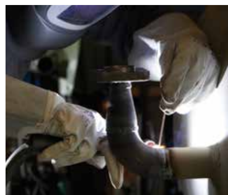
The Focus TIG 200 DC HP PFC welds mild and stainless steels and other DC-weldable materials
